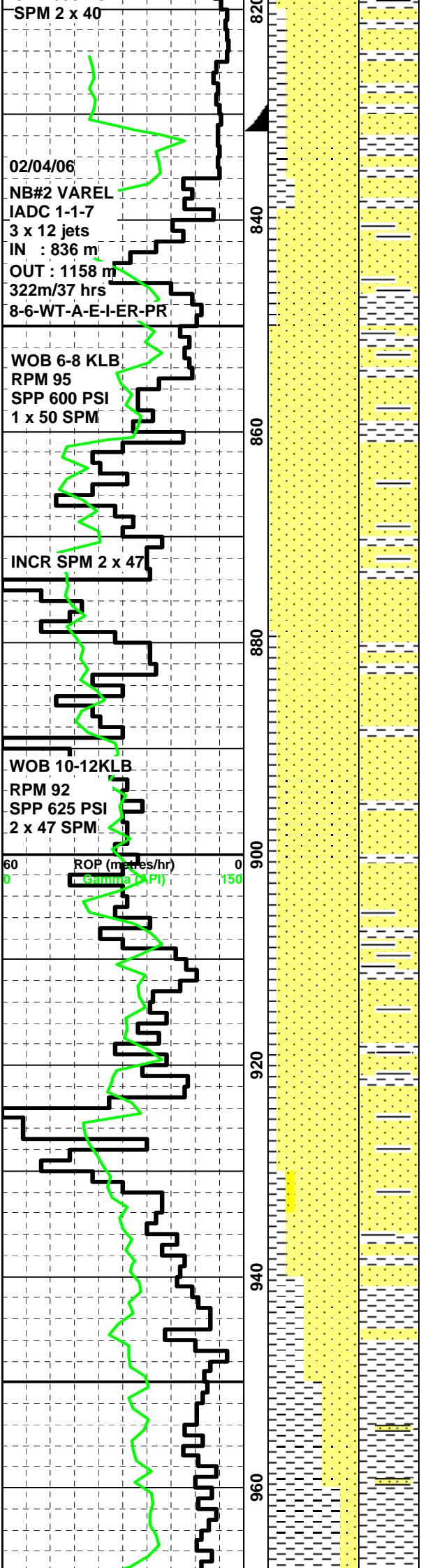
DRILLED 12-1/4" HOLE TO 836 m
