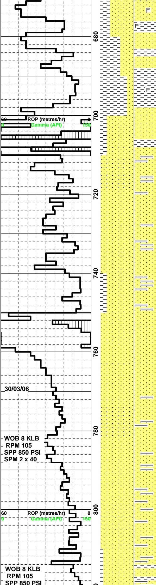
CLAYSTONE: m brn gy- occ m gy, v sft-occ frm, amorph-subblk, stky, silty i/p, tr qtz gr, calc, occ carb, tr pyr, Note: sample washing out
