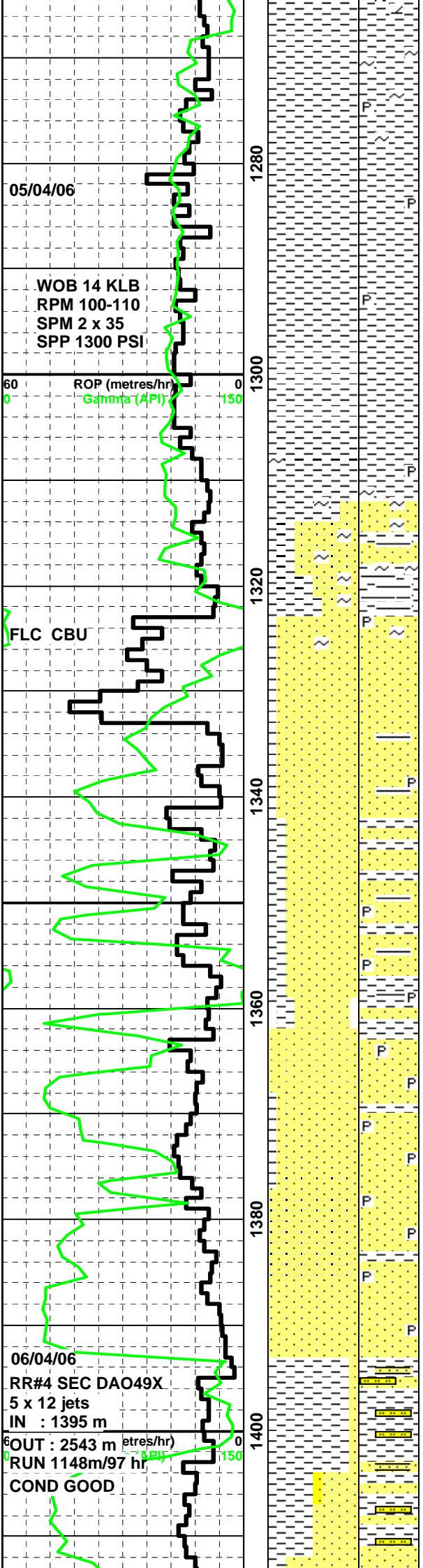
**CLAYSTONE**, m gy brn- v dk gy, frm, sbfiss, rr-tr glau, sl carb i/p, calc, occ v thn lam of qtz siltst, tr carb f-m ssd, tr dol a/a, grdg i/p to carb shale & silty Claystone
