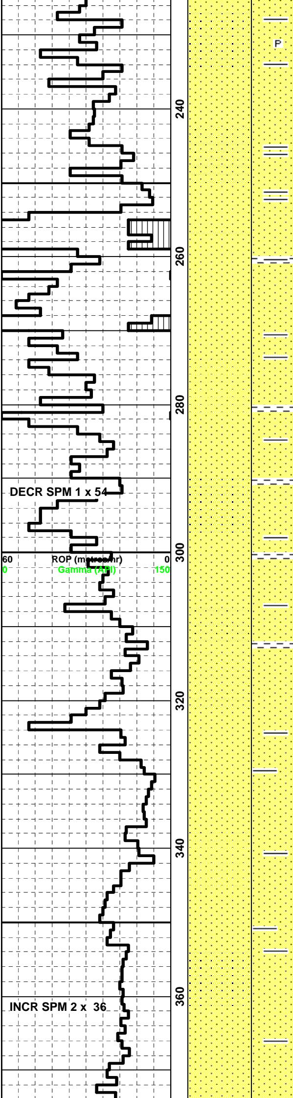
SANDSTONE: clr-v lt gy-occ wh, transl-occ opq, vf-crs dom f-m, subang-subrnd, mod srtd, com-abnt lse mica, tr wk sil cmt, gen lse-unconsol, tr blk coal mtl, tr brn arg mtl, fr inf por
