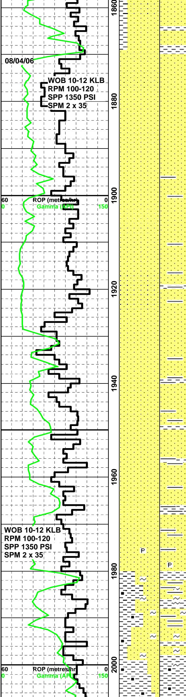
NOTE: SHAKERS BLINDING - POOR SAMPLE RECOVERY
